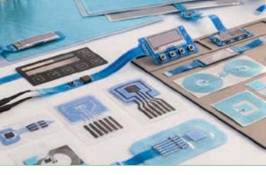
Printed circuitry, heating elements, membrane switches, user interface graphics, conductive paths, and traceable labels on flexible or rigid substrates.            | Printed heaters, conductive circuits, biosensors, RFID/NFC antennas, digital dose/therapy counters, touch controls, shielding layers, smart packaging sensors.  |
